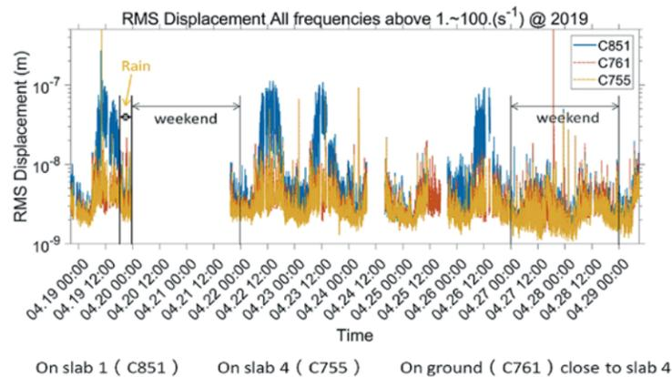
The vertical ground motion measurement results on HEPS ground and the two prototype slabs: the red line shows the motion on ground, the blue line shows the vibration on prototype slab #1 with 1m graded sand gravel and 1m reinforced concrete, the yellow line shows the vibration on prototype slab #4 with extra 5m casting layer.
