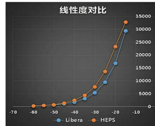
Linear measurement data of digital BPM electronics (home-made vs Libera)
